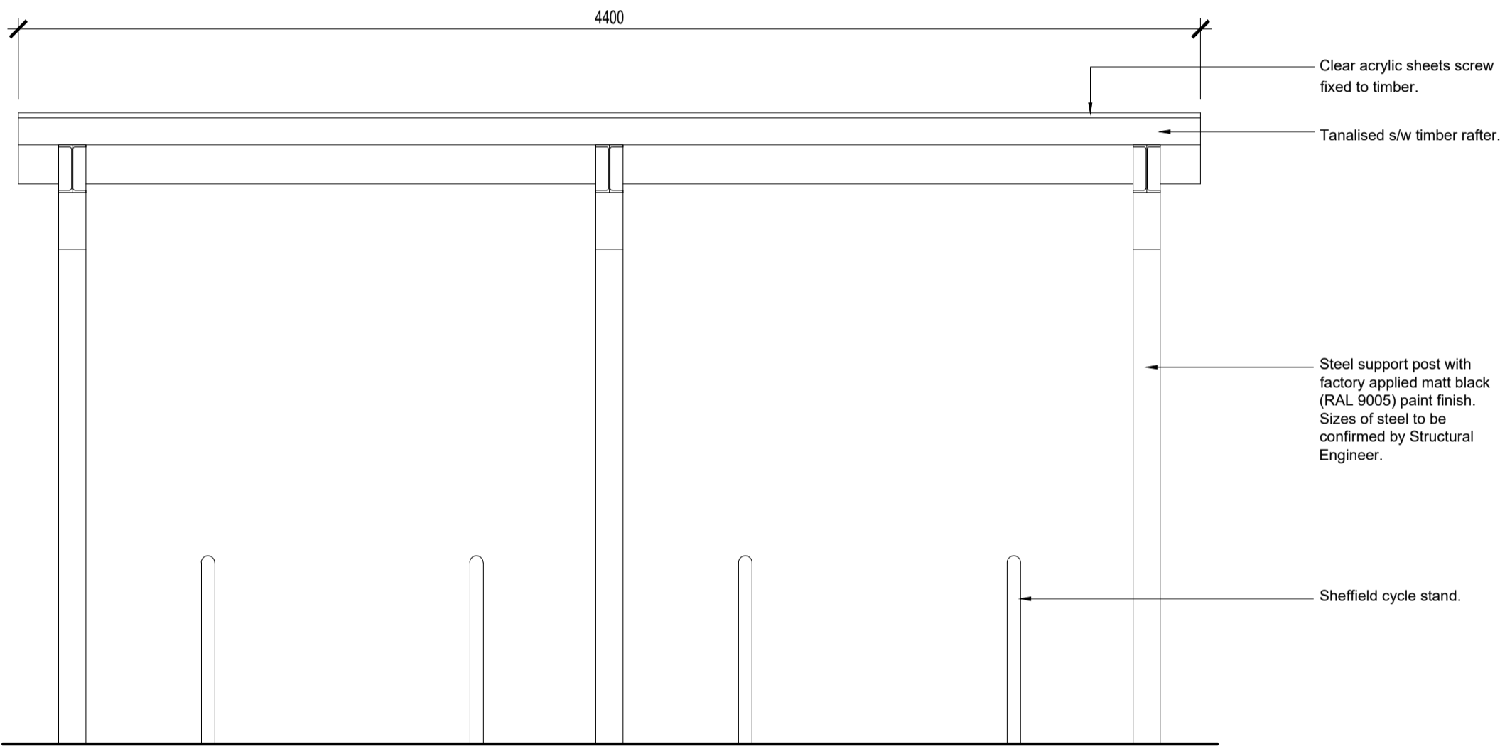
Covered Cycle Storage - Elevation A (Front) Scale, 1:20
